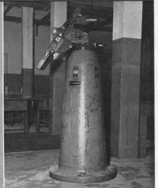
Typical of Canadian skill and ingenuity in the saving of critical materials, are the new open-type Oerlikon anti-aircraft gun mounts which are now being delivered from GM at Oshawa. Illustrated, above, is an old-type solid mount compared with the new metal-saving open-type mount which is now rolling from the GM lines.
